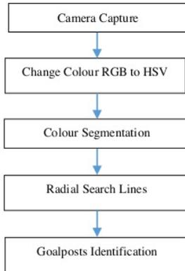
Figure 6. Goal Detection Process Diagram
