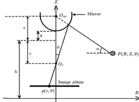
Figure 4. Hyperbole omnidirectional mirror model
