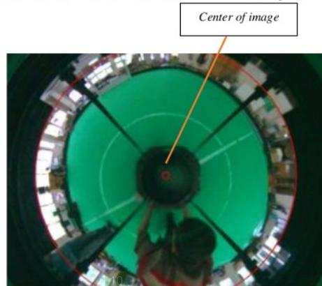
Figure 10. Determine the center of the omnidirectional camera image
