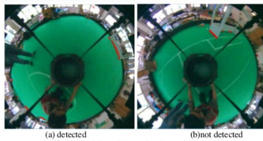
Fig 12. Goal detection result using radial search lines
